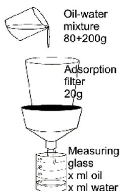
Figure 21. Oil adsorption filter and test equipment.
