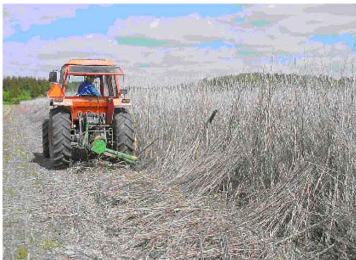
Figure 17. Cutter bar mower used in the spring cutting of hemp fibre on Suitia experimental farm in May 2001.
