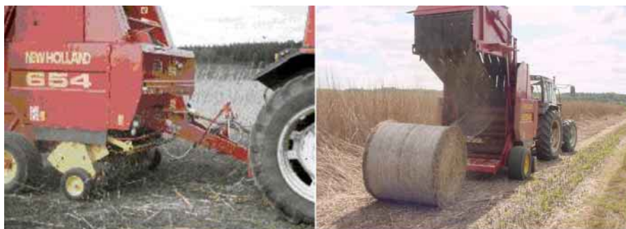
Figure 18. Harvesting hemp fibre with a round baler on the Suitia experimental farm in May 2001.
