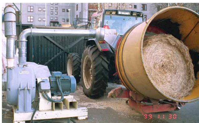
Fig 19. The “Tomahawk” straw chopper (right) combined with a hammer mill (left) as a round bale opener is tested in Viikki in the autumn of 1999.
