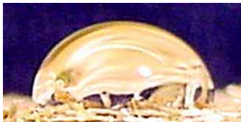
Figure 24. Large contact angle of a water drop on a pressed tablet.
