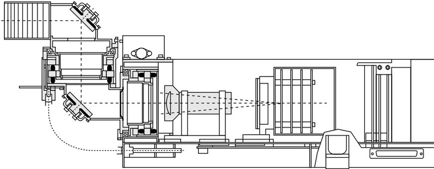
Figure 2.1: Schematic representation of a SWAN sensor unit. After Bertaux *et al.* (1995).
